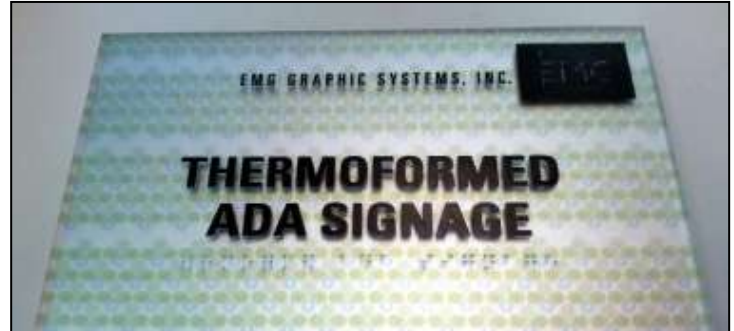
Translucent ink pattern on clear vinyl is encapsulated between two clear 1/8" acrylic sheets. Back painted using a silver metallic Matthews Acrylic Polyurethane. Cut, cleaned and tipped to create multiple visual planes within a monolithic structured sign.
